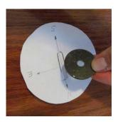
3. The<u>n</u>, they 'magnetized' the paperclip by rubbing a magnet along it. They rubbed the magnet south TO north, and make sure you only go in one direction.
